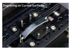
Engraves on metals with curved surfaces such as bracelet, pen, hip flask, and ball.
