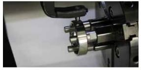
• Engraves patterns, letters or names on the inside or outside of a ring using two separate embedded tools.
